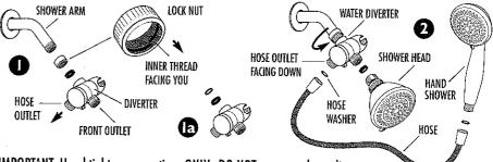
IMPORTANT: Hand tighten connections ONLY. DO NOT use wrench or pliers.
