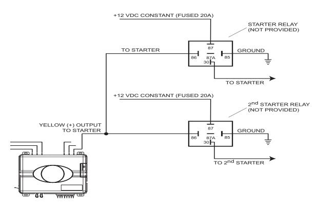
**note!** Always check the Web site information on your vehicle for warnings regarding the starter wire and check engine lights. Some vehicles will trip a check engine light if the starter wire is cut.
