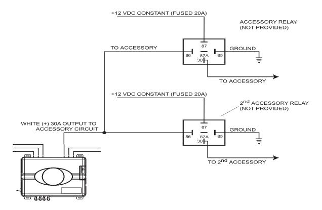
If your vehicle requires more than one accessory then the GREEN ign2 wire can be programmed to function as an accessory output.
