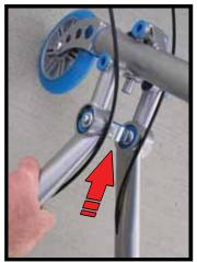
Insert the main axle through the 3 main frame parts and tighten the bolt with the 5 mm allen wrench.
